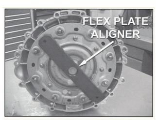
Note: V-8 models the flywheel must be aligned properly to the torque converter.
