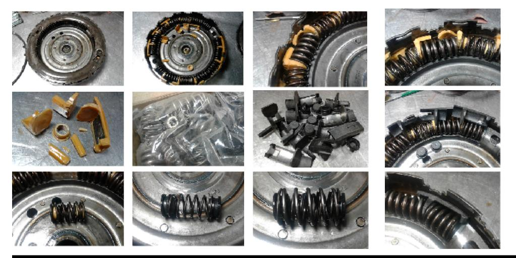
The use of repair kits eliminates bumps when switching gears, restores the comfort of driving. The quality of repair is confirmed by mandatory road tests. The characteristics of the restored damper disk correspond to the parameters of the new one, which allows to save considerably on its replacement.
